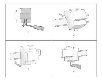
To unmount the device, make sure to unplug the network connection and the bus terminal from its housing. Use a screwdriver to slide down the lock and remove the device from the rail.
