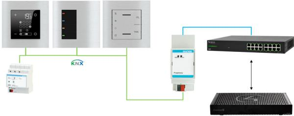
This specific functionality does not require any configuration in KONNECT4, and can be easily reached with a standard KNX communication driver offered by Control4.
