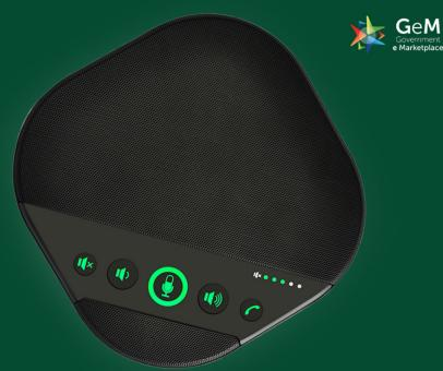
4 Unidirectional HD Microphone Array USB 2.0, Bluetooth & AUX I/O Interface Built-in Li-ion Battery
